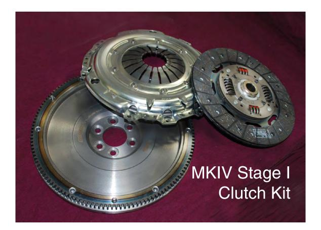
The **ECS Tuning Stage I** clutch kit is a lightweight replacement for the factory-installed VW MKIV dual mass flywheel. The single mass flywheel conversion kit bolts directly to the crankshaft without modification, and comes with a mating clutch package that includes friction disc, pressure plate, release bearing, and pilot tool, plus new flywheel and pressure plate bolts.
