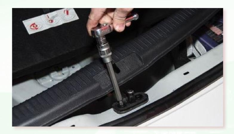
Slide the lock post towards interior of the car 3-5mm. Re-tighten and close the hatch for test fitment. Adjust until the desired position is found.
