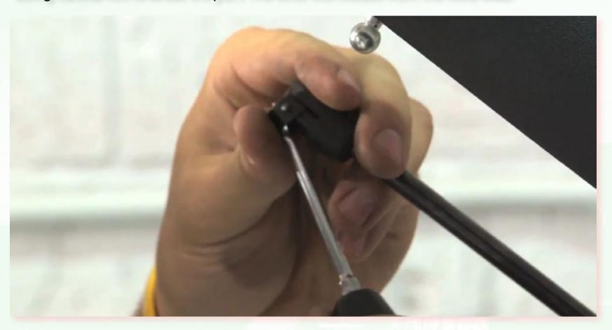
To remove the existing mounting stud, use a 13mm wrench. The procedure for replacing the strut and mounting stud is identical for the left and right assemblies.
