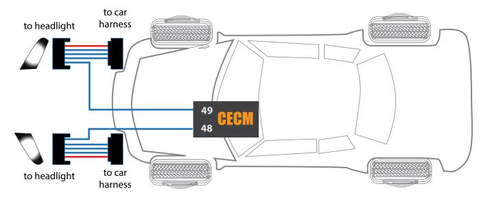
This schematic shows the general location of the connector harnesses. The long blue wires from the harnesses run into the vehicle through the firewall and connect at termnals 48 and 49 of the Central Electronics Control Module beneath the dash.
