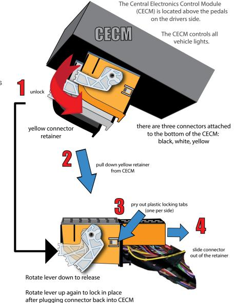
Pry on the locking tabs (step 3) and slide the wiring connector with wires out of the plastic retainer. HID (High Intensity Discharge) Headlight Conversion Harness Kit Installation
