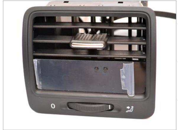
**3** Insert the slats assembly into the vent, lining up the tabs and slat controller, it will fit snugly. Feed the wire through as shown, you may need to kink the wire at a 90 degree angle to keep the wire in place. Line up the glass onto the vent, press to adhere it to the front of the vent frame as shown. After you verify the gauge is fitted as shown, slide on the front of the vent until all 4 clips click into place.
