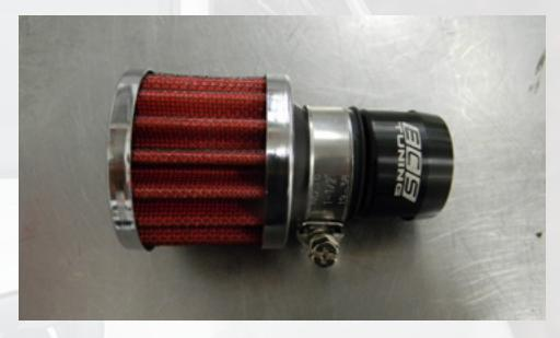
Step 12 Insert the secondary air pipe adapter into the air pipe filter and tighten the clamp.
