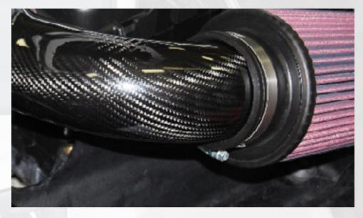
Step 18 Install the 3" straight coupler onto the end of the mass air flow sensor.
