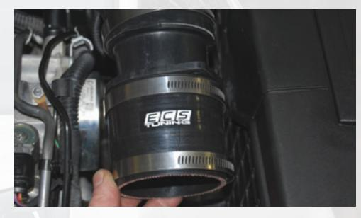
Step 20 Insert the carbon fiber air filter tube into the 3" straight coupler.
