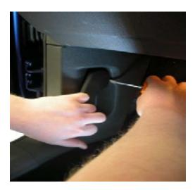
2.) Using the flathead screwdriver, gently pry off the cap covering the screw head on the driver's side hood release panel. Once this is removed, use the flathead screwdriver to remove the securing bolt you have just exposed.
