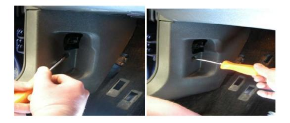
3.) After removing the flathead securing bolt, gently pry up on the driver's side plastic door sill to allow room for removal.
