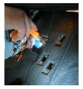
7) Take the R32 Dead Pedal, and gently slide it down into the holes in the floor. (Only two of the three OEM retaining holes are used with the ECS Dead Pedal, the third will remain unused)
