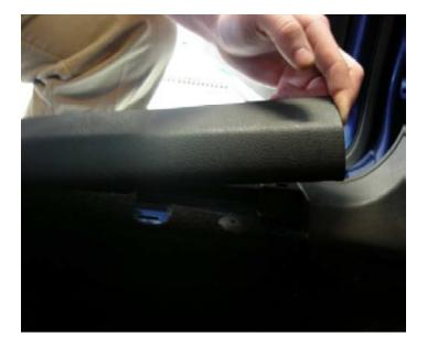
12) Remove the plastic covering from the dead pedal, exposing the plastic finish. We recommend you do this step last, to prevent the tools from possibly scratching the finish during install.
