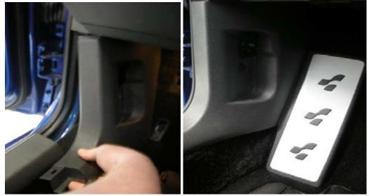
10) Take the plastic securing clip for the hood release handle, and re-insert it as shown in the picture. Make sure it clips into the handle, and is seated completely. After this is done, take the hood release handle, and place it back onto the car by pushing it until it "pops" into place.
