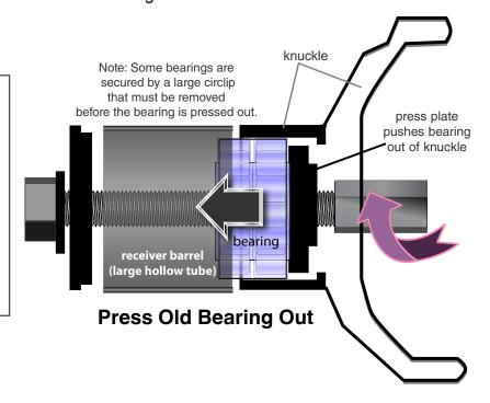
Note: Press tool and receiver barrel sizes are selective. User discretion is required to ensure that the correct diameters are used.
