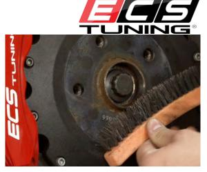
Clean the hub collar and face and the mating surfaces on the wheel.
