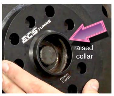
Thicker spacers center on the wheel hub and add a raised hub of their own to keep the wheel centered. Never install a hubcentric wheel without a raised centering collar.
