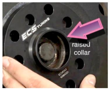
Thicker spacers center on the wheel hub and add a raised hub of their own to keep the wheel centered. Never install a hubcentric wheel without a raised centering collar.
