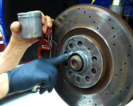
Apply a thin film of antiseize compound to the hub face. This will help prevent rust, and make hub removal easier at a later date.
