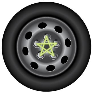
Tighten lug bolts in steps using a star pattern.
