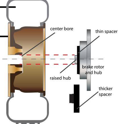
2) Use hubcentric spacers when necessary. Hubcentric wheel hubs have a raised center that engages the wheel center bore. This keeps the wheel centered on the hub.
