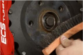
Clean the hub collar and face and the mating surfaces on the wheel.
