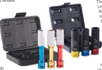
17 mm for VW/Audi oem bolts (19 and 21mm for non-oem aftermarket applications) The Schwaben Torque-Limiting Wheel Bolt Socket Set prevents over-tightening of wheel bolts and lug nuts. Attach them to your ½-inch impact gun and tighten the wheel bolts or lugs until the socket stops tightening at 74 ft-lb (100 Nm). Then final-tighten the wheel fasteners to the recommended tightness using a torque wrench.
