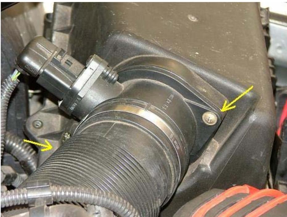
Next, remove the two phillips screws that hold the mass airflow sensor to the air box lid. Set the air box lid and filter aside.
