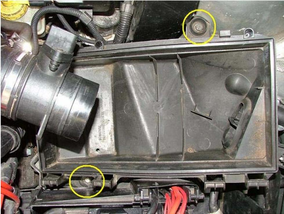
Remove the bottom half of the air box by removing the two 10mm bolts that secure it in place.
