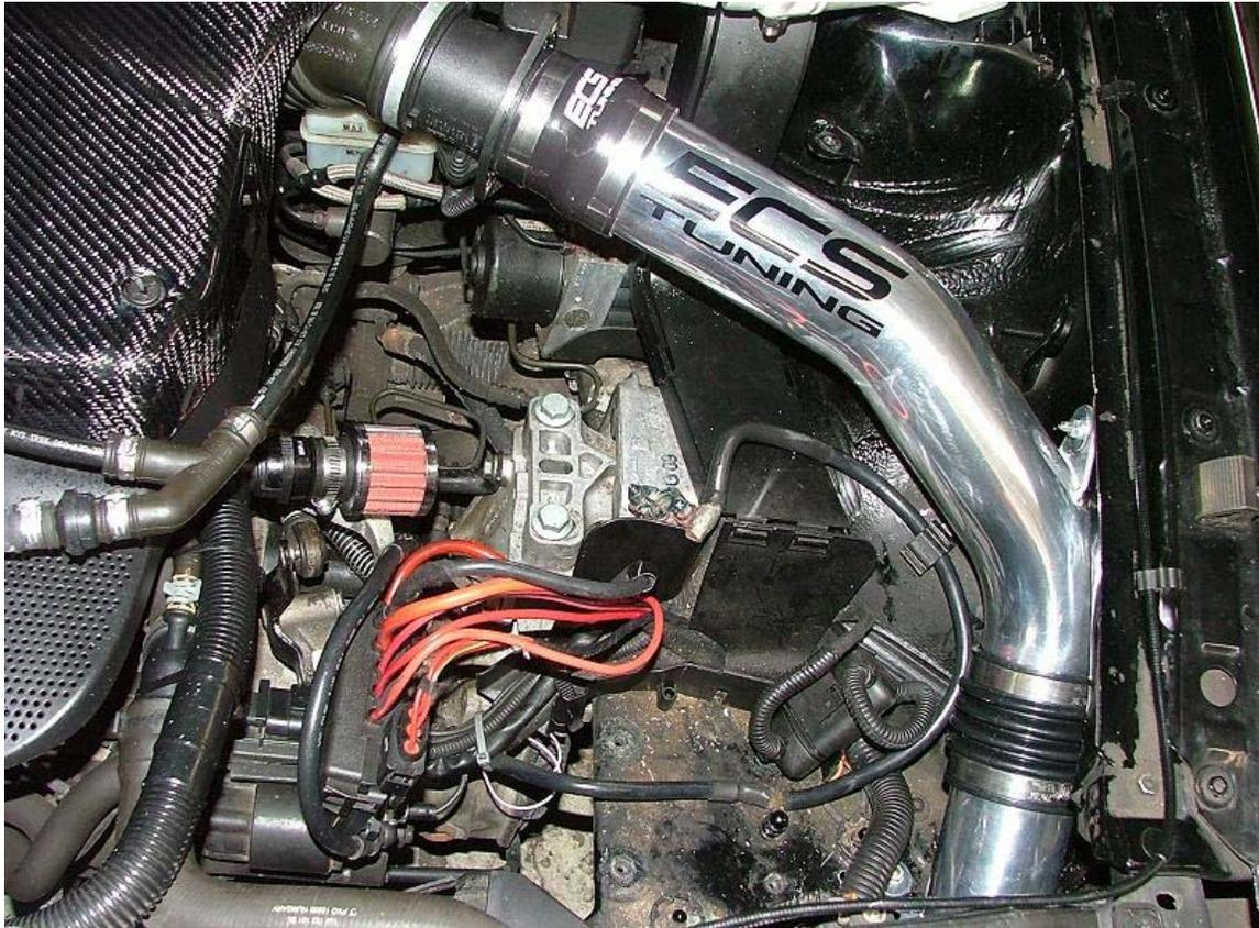
Attach the intake pipe to the mass air flow sensor using the supplied silicone hose connector and 3" clamps. Installation note: Loosen the top flex section clamp while fitting the intake. This will allow for the best possible fit on your vehicle. Once satisfied with mounting position, tighten the clamp to further secure the intake.
