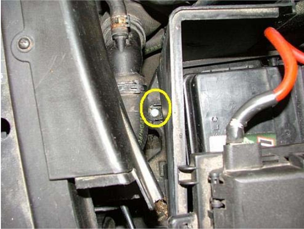
Remove the 10mm bolt holding the battery cover, remove the battery cover and set it aside. Installation note: Battery, and battery tray can be removed. While not necessary, removal of these components allows for more room to work, resulting in an easier installation. Also, disconnecting the battery may require you to re-enter your radio anti-theft code.
