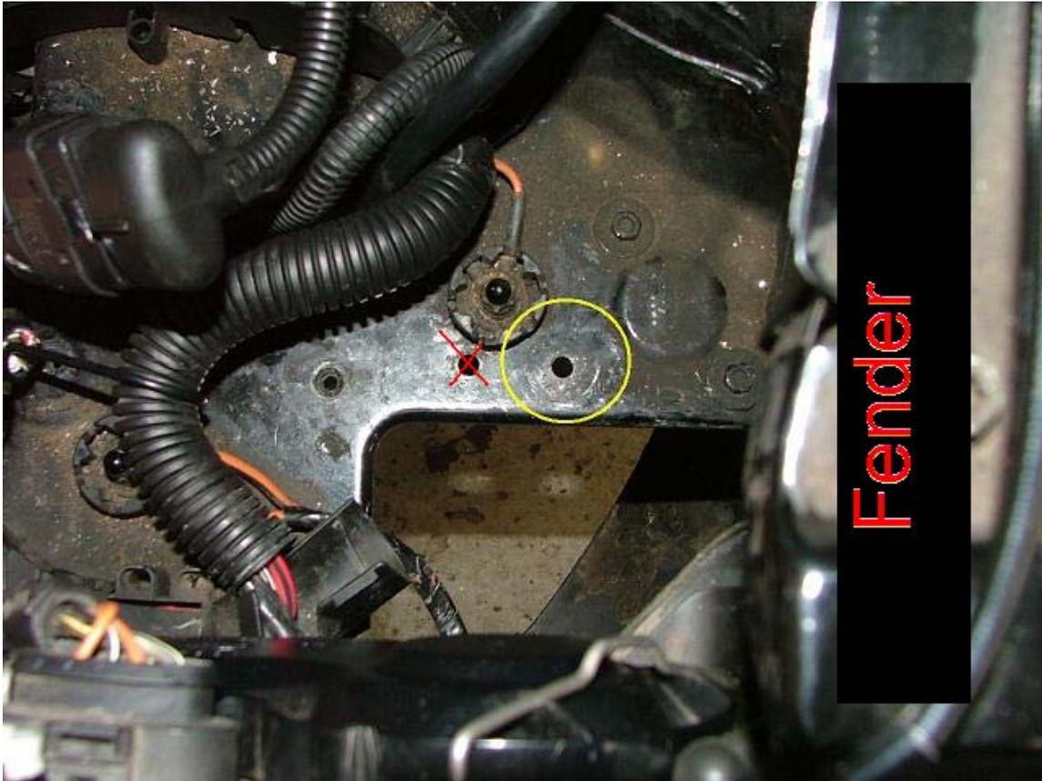
When mounting the intake to the lower fender well, the correct pre-drilled hole must be used. ALWAYS USE THE HOLE CLOSEST TO THE FENDER.
