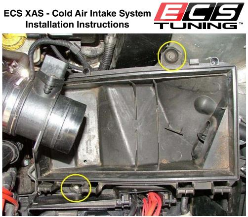
Remove the bottom half of the air box by removing the two 10mm bolts that secure it in place.
