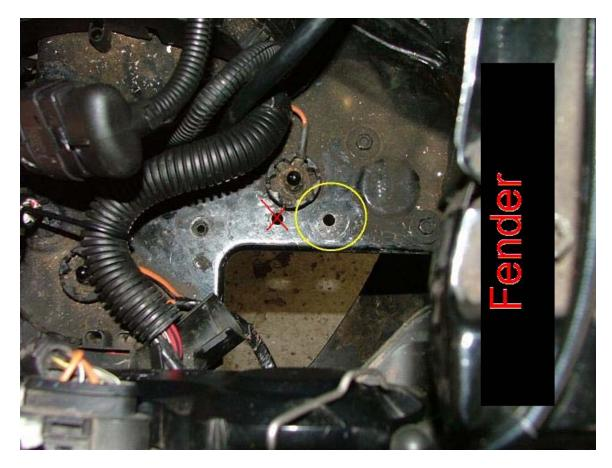
When mounting the intake to the lower fender well, the correct pre-drilled hole must be used. ALWAYS USE THE HOLE CLOSEST TO THE FENDER.
