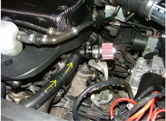
Using zip ties, Secure the breather filter out of the way of all shifting and radiator components.
