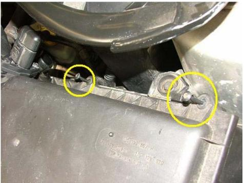
Begin the installation by removing the two phillips screws that secure the air box lid.
