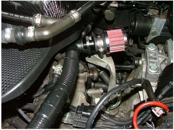
Clip the supplied adapter with supplied attached into the female breather tube that was previously connected to the back of the air box.
