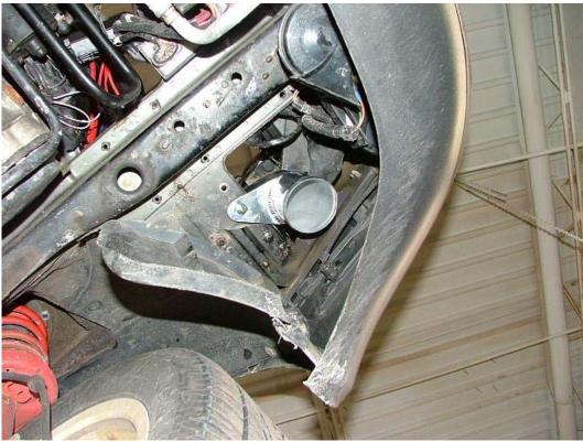
Using the supplied double male rubber mounting brace, attach the intake to the lower fender mounting location.
