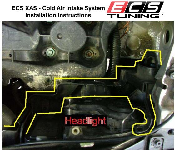
To get the air duct guide (out lined) out from underneath the headlight, you must take a 13mm socket with a 10" extension and remove the front battery hold down bracket. The air duct guide is held in place with 3 plastic rivet type pins, these pins are in locations difficult to reach. Removal of air duct guide with out removing the pins will probably result in broken pins or air duct guide.
