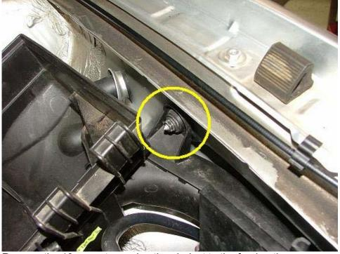
Remove the 10mm nut securing the air duct to the fender, then remove air duct.
