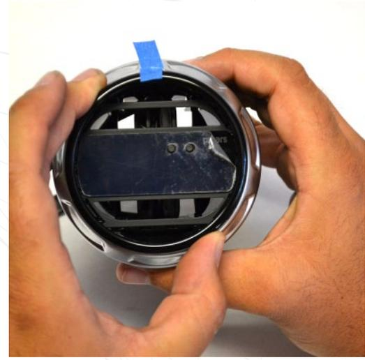
Line up the inner trim ring with the markings that we placed in step 1. Gently insert the ring with no force to get it lined up and seated but not yet clicked into place.
