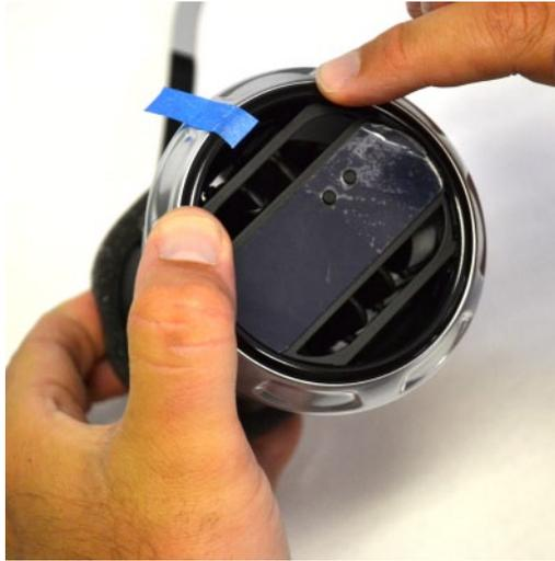
Apply pressure to the top clip locations as shown to seat the top clips.
