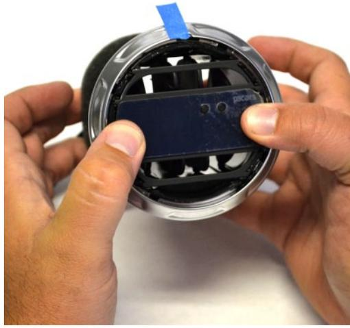
Line up the tabs of the metal display bracket to the vent slat positions. Center the gauge perfectly before applying pressure evenly to the sides of the gauge as shown.
