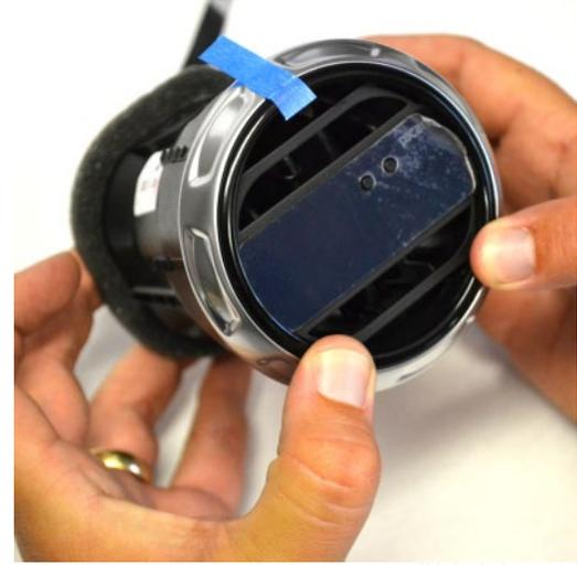
Apply pressure to the bottom clip locations as shown to seat the bottom clips. After the clips are seated you can remove any center markings you applied.
