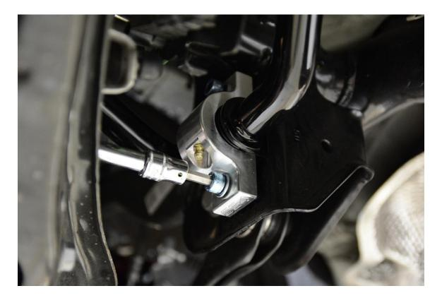
**Step 9** – Verify that the Solid Rear Sway Bar is installed correctly, then (if you unbolted it) reinstall the level sensor bracket and level sensor to the lower control arm using the T25 screws.
