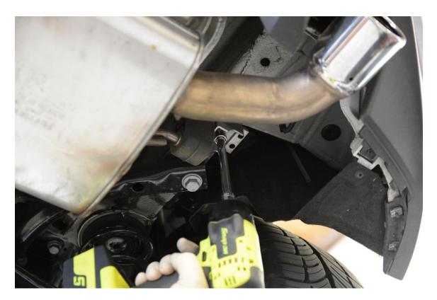
**Step 5** – (Optional) In order to give yourself more room to work with, remove the T25 screws attaching the level sensor to the lower control arm. **Carefully** remove the factory rear sway bar.
