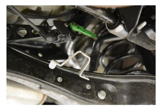
**Step 6** – Grease and reinstall the supplied Polyurethane Sway Bar Bushings onto your 034Motorsport Solid Rear Sway Bar Upgrade as shown below. **Carefully** install the 034Motorsport Solid Rear Sway Bar.
