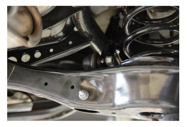
**Step 8** – With the sway bar properly aligned, install the supplied Billet Aluminum Sway Bar Mounts with the zerk fitting pointing down. Secure using the supplied M8 Bolts & Washers. Torque to 28 Nm.
