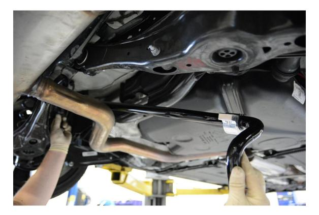
**Step 7** – With the sway bar in place, reinstall the nuts to the factory rear end links, or install your new MQB Spherical Rear Sway Bar End Links if you purchased those as well. Torque the stock hardware to 35 Nm.
