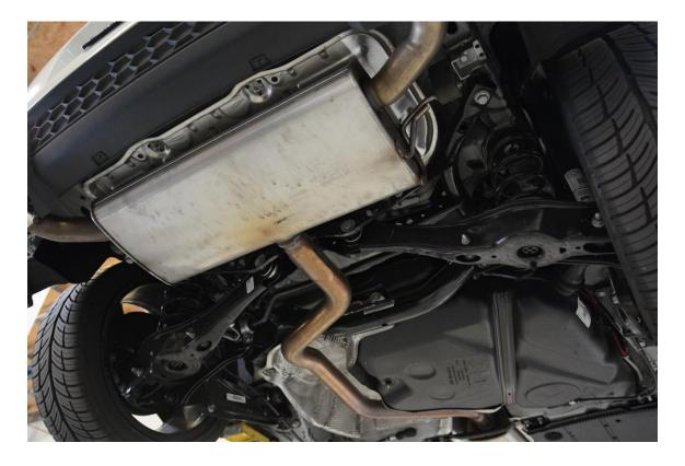
**Step 2** – Using the 10mm Triple Square, remove the two M8 Bolts securing each of the factory rear sway bar mounting brackets to the subframe.
