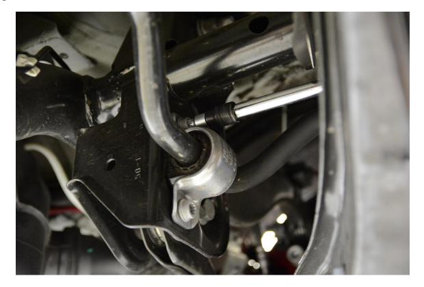
**Step 3** – Using a 16mm wrench and 6mm triple square, remove the nut securing each of the rear sway bar end links to the rear sway bar.
