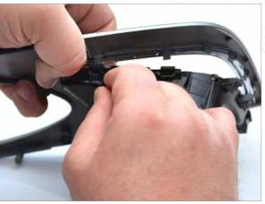
Using a flat blade screwdriver, unclip the trim from the vent, be careful that the slats do not fall out.
