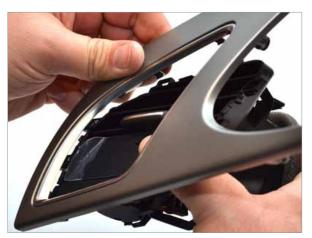
8 Carefully re-attach the trim to the vent assembly. If you have trouble keeping the parts from falling out, you can use a temporary piece of tape across the right side to hold them in until the trim is in place.
