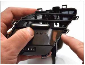
Peel the protective covering off both sides of the glass face so the tabs are not covered. Insert the tabs on the glass into the holes on the vent as shown here starting with the far side. The gauge should rest inside the slots where the vent slates were before. If the gauge will not sit flush, check that the wire is positioned properly.
