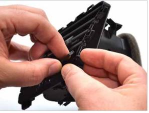
Carefully remove ONLY the bottom slat starting on the side of the vent that is closest to the steering wheel.
