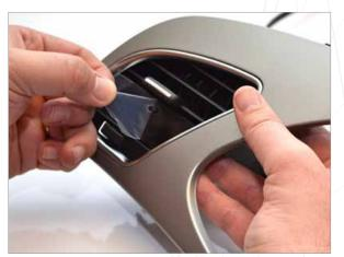
9 Peel the remaining protective covering off the gauge and it is ready to go back into the car. Follow the generic "in car" instructions for the remainder of the install.
