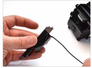
Prepare the display unit, make sure the wire comes off the back at a 90 degree angle.
