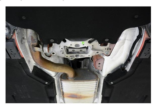
**Step 2** – Using a 10mm Triple Square, remove the two M8 bolts securing the factory transmission mount bracket to the transmission mount assembly.
