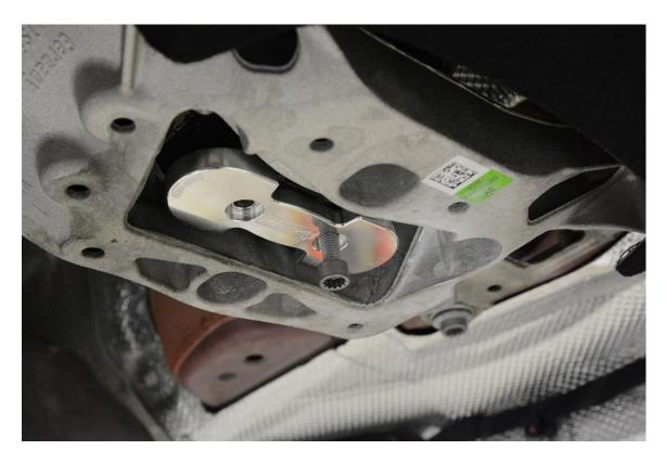
**Step 5** – Torque the factory M8 bolts to 25 Nm with Blue Loctite applied. Make sure to thread in both bolts before tightening either of them to spec to ensure that the insert is properly lined up.
