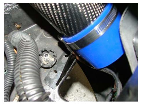
Position the lower support bracket as shown in the above picture and bolt the bracket to the lower fender.
