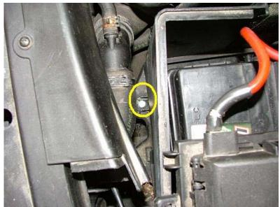
Remove the 10mm bolt holding the battery cover, remove the battery cover and set it aside. Disconnecting the battery may require you to re-enter your radio anti- theft code.
