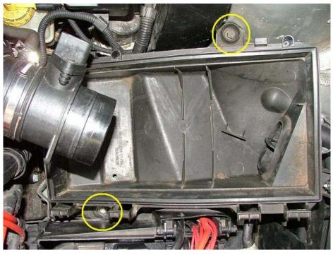
Remove the bottom half of the air box by removing the two 10mm bolts that secure it in place.
