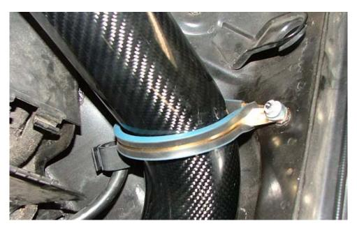
Install the supplied cushioned loop clamp as shown.
