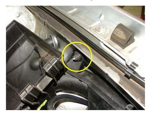
Remove the 10mm nut securing the air duct to the fender, then remove air duct.
