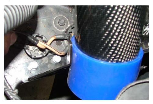
The above picture shows the bracket installed, and the intake positioned against the bracket. Install the clamp around the notched part of bracket and silicone coupler to secure lower half of intake.
