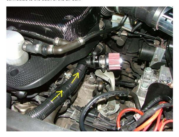
Using zip ties, Secure the breather filter out of the way of all shifting and radiator components.
