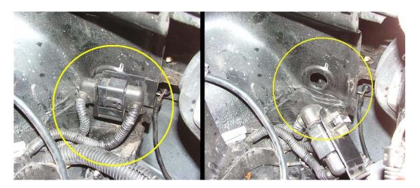
To ensure intake pipe clearance, the clip must be removed from the inner fender. Once removed, tuck it to the side.
