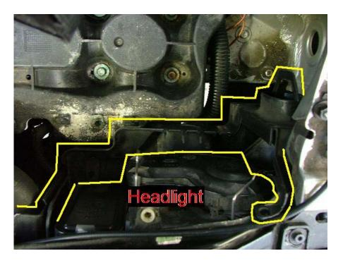
To get the air duct guide (out lined) out from underneath the headlight, you must take a 13mm socket with a 10" extension and remove the front battery hold down bracket. The air duct guide is held in place with 3 plastic rivet type pins, these pins are in locations difficult to reach. Removal of air duct guide with out removing the pins will probably result in broken pins or air duct guide.
