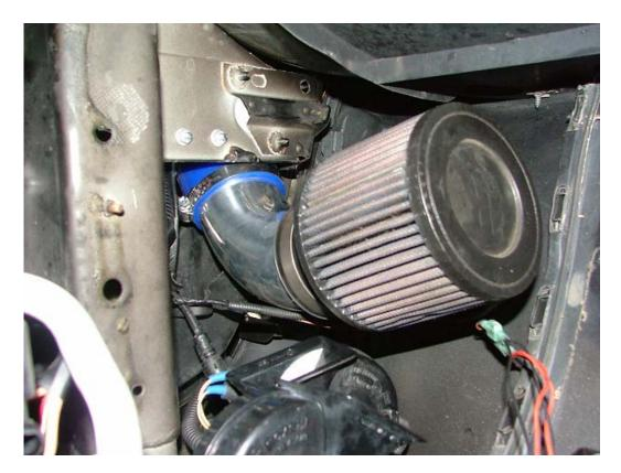
Attach the High Flow Intake Filter to the end of the intake Pipe
