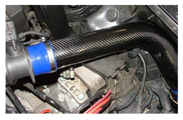
Attach the intake pipe to the mass air flow sensor using the supplied silicone hose connector and 3" clamps. Once satisfied with mounting position, tighten the clamp secure the intake.
