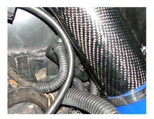
Tuck connector out of the way, behind the intake pipe as shown.
