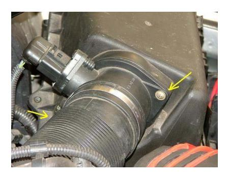
Next, remove the two Phillips screws that hold the mass airflow sensor to the air box lid. Set the air box lid and filter aside.
