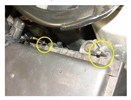
Begin the installation by removing the two Phillips screws that secure the air box lid.
