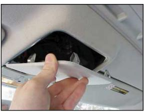
e. Disconnect harness from light panel. Use a screw driver to free each side of the plug.
