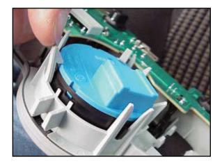
g. Install the old knob into the new W8 light panel. Note the orintation of the black/blue/black tab on the switch; It should face the bulb sockets in the panel. Before seating the switch, flip the panel over and check that the knob rotates correctly withing the markings on the panel.
