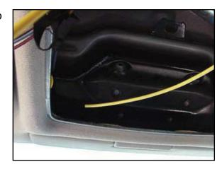
j. Continue to run the wire down the A-pillar to the headlight switch. You can use a credit card or simillar to tuck the wire between the glass and cover, this actually works very well. (The A-Pillar cover can be removed to better hide this wire.)
