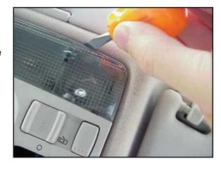
b. The lens will simply flip down and pull out.
