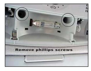
d. Remove the cover from the sunroof motor compartment. This is held in with just simple spring clips. Pry down with your thumb, using screw driver may help here.
