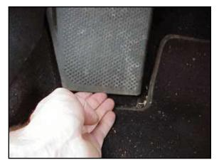
e. Note the clip on the left hand side of the Dead Pedal and how it clips into the lower left kick panel. Noting this will simplify removal and re-installation.
