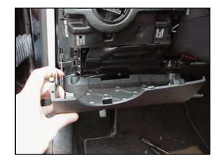
d. Remove the single torx screw from the top of the Dead Pedal. Slide the pedal up and then twist the right side towards you to remove.
