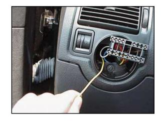
g. Pull the wire down in front of the hood release lever. With the dead pedal removed you will be able to pull up on the kick panel to help feed the wire thru.
