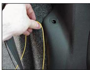
n. Feed the wire up under the rear deck hatch trim piece. Push at least one foot of the wire up under the trim.
