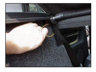
p. Run the remaining length of wire behind the CD bracket and carpet.
