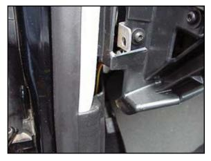
h. Continue running the wire down the running board. A small screw driver and credit card work well here. You can optionally pull the running board up, but is not necessary.
