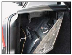
q. Disconnect the tail light and remove the bulb assembley by squeezing in on the to retaining clips.
