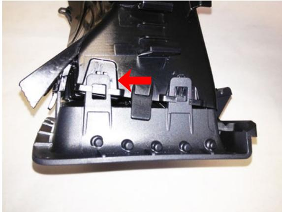
**3** Repeat the clip releasing procedure on the sides and bottom of the vent.
