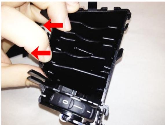
**5** Using your fingers flex the top of the vent upwards to release all of the inner vertical slats of the vent. After all inner slats are removed set them aside in a safe place in case you wish to return your vent to stock.
