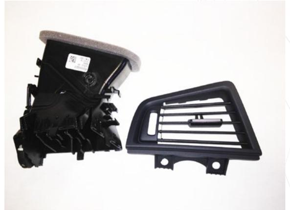
**4** Work your way around the vent releasing all clips until the front face of the vent is free.
