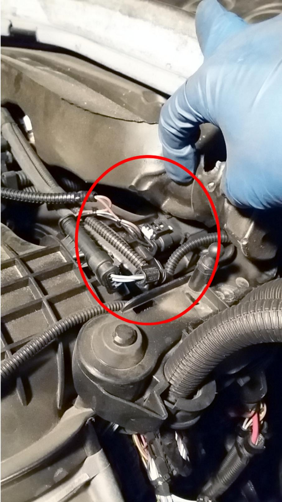
5) Fuel Pressure Connector, black patch. Optional to install.
