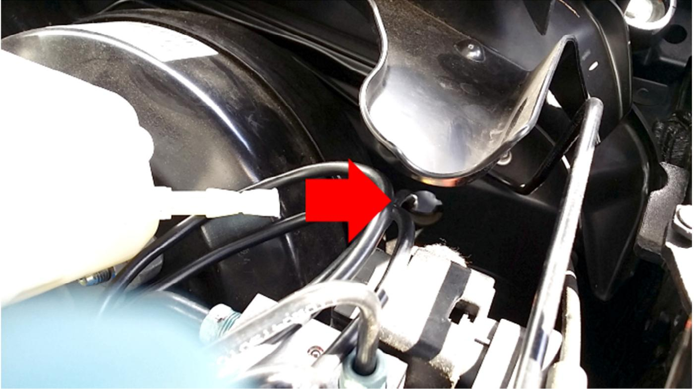
Note those with a manual transmission have the clutch line run through this same hole. You'll need use a coat hanger to pull CANbus wire around the grommet. Alternatively you can use cut a small slide in the grommet to facilitate feeding the CANbus wire through.
