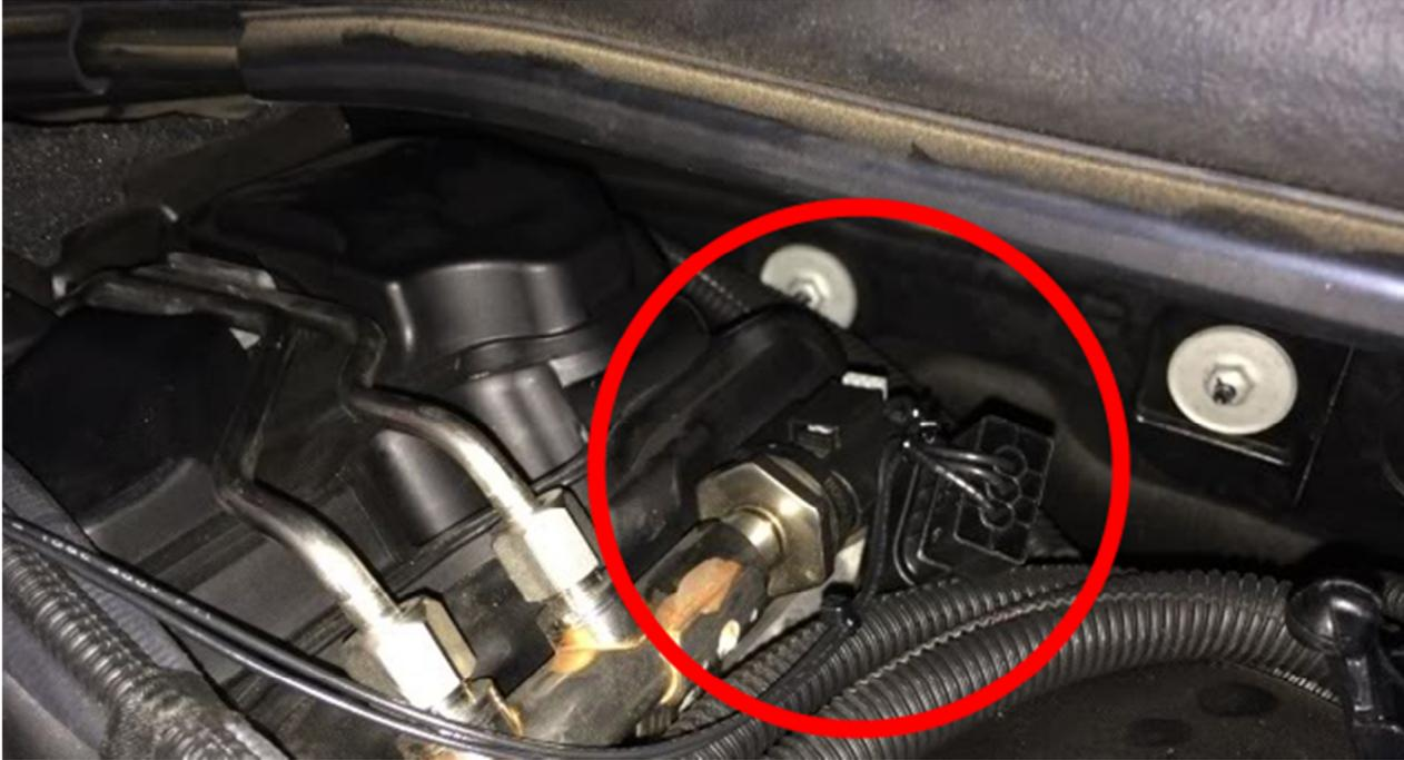
6) Boost solenoid, blue patch: Pneumatic Wastegate Vehicles Only.
