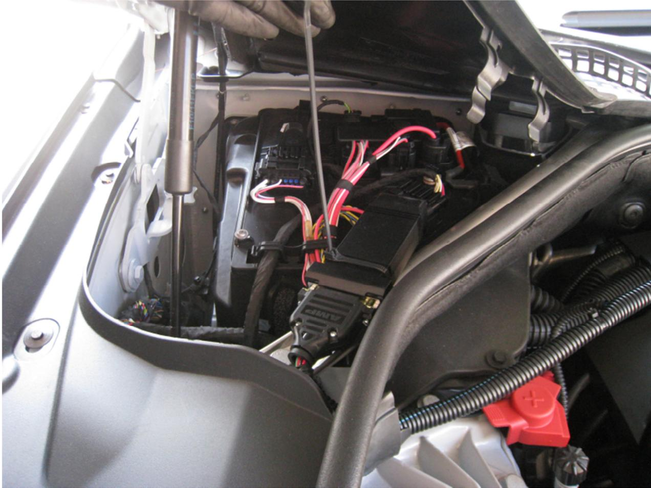
TMAP ground bypass required if USB cable touches battery rail, install wires with battery connected, etc. If you get a check engine light with the tuner completely removed you likely damaged the TMAP ground and need to perform this step to repair it. POSI-TAPS are on our website. While this is the quickest & easiest fix more detailed directions are posted to n54tech to repair the TMAP ground trace directly.
