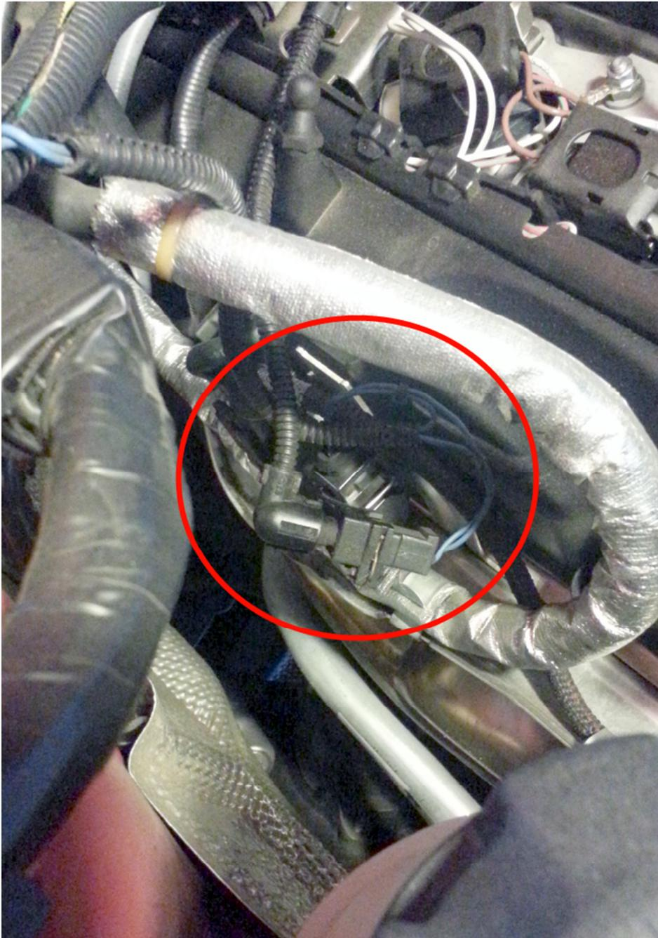
7) OBDII CANbus -- Required for in dash map switching via BC button, CANflap, datalogging, and all other in dash features. If you fail to install this connector the JB4 will act as if its on map1 (default map) regardless of what map is selected.
