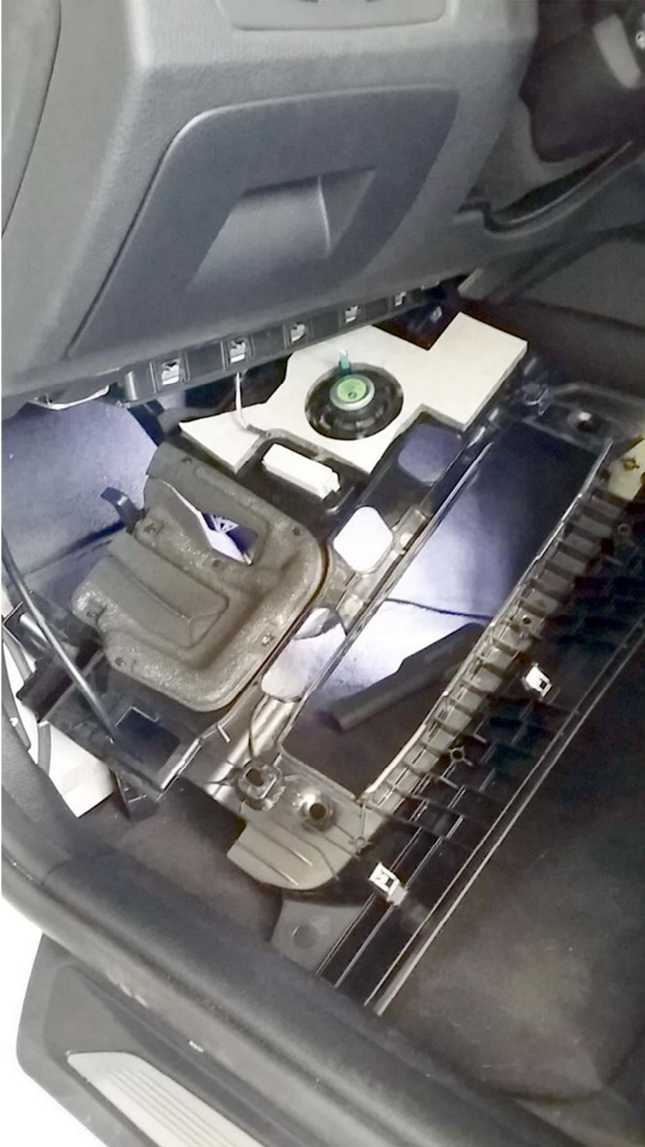
Using a long screwdriver push in on the rubber firewall cap pushing it in to the interior compartment. You'll see it fall down by the pedals and can put it away for safe keeping. Feed the OBDII wire from the interior through the hole to the engine compartment. Note 535 models have a foam cover that is pulled off to access the rubber plug.
