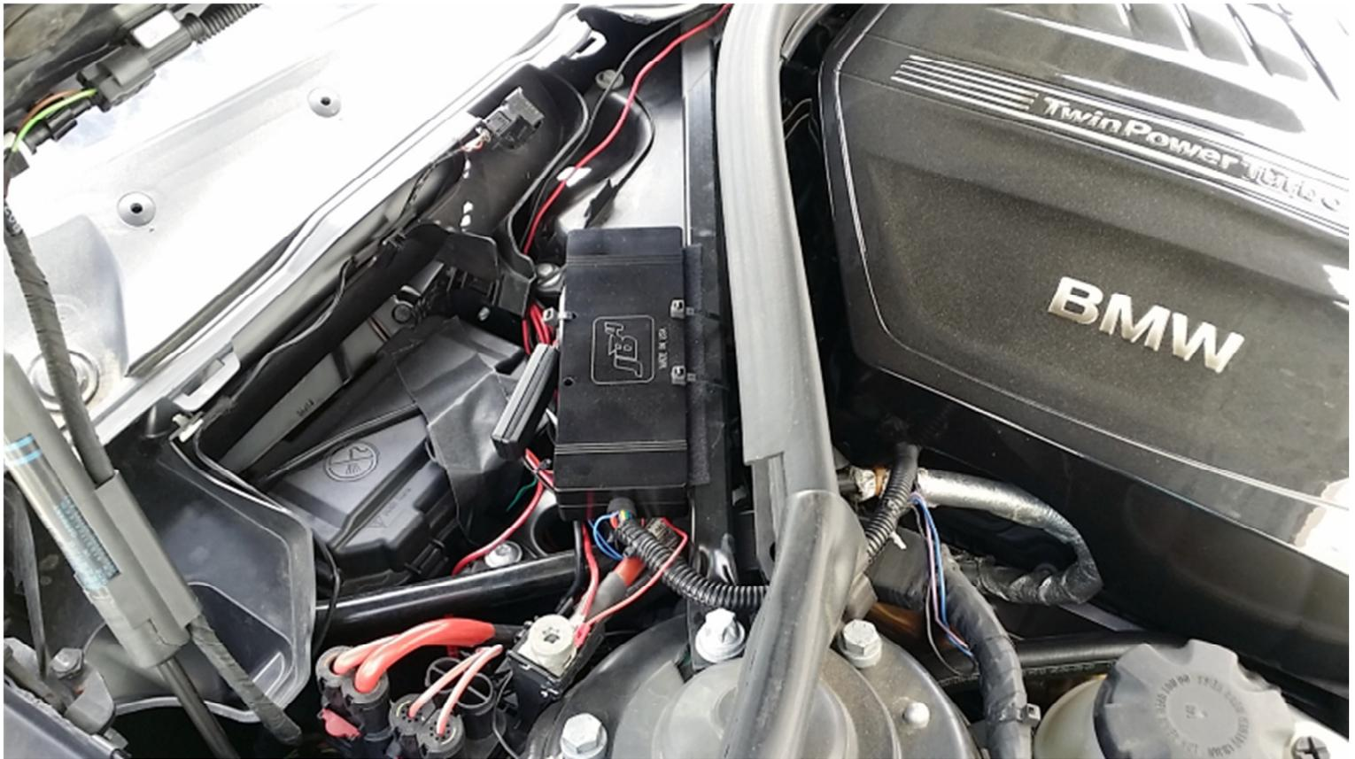
When reinstalling the cowl cover be sure it's fully seated and that you've lifted the rubber seal around it.
