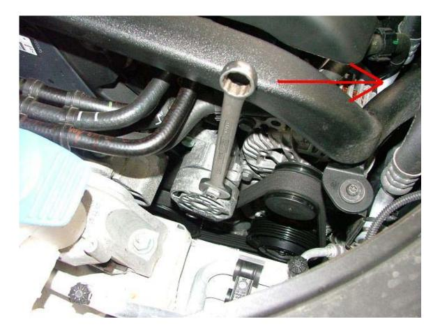
Next, remove the stock belt using a 16mm combination wrench to release tension as indicated in the above picture.
