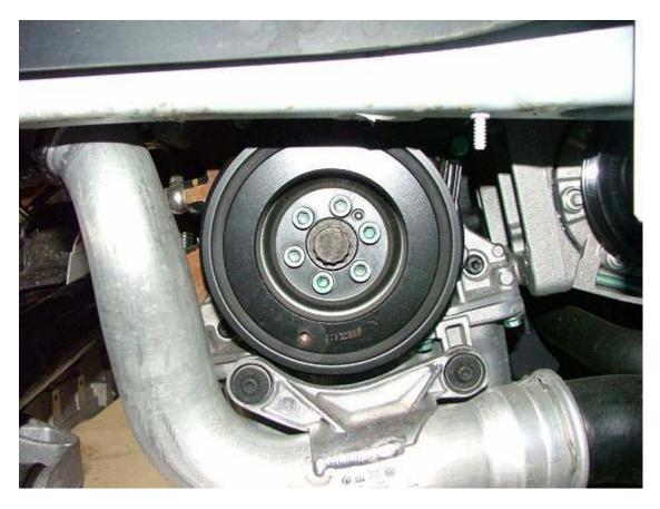
Remove (6) 6MM Hex bolts holding stock crank pulley.
