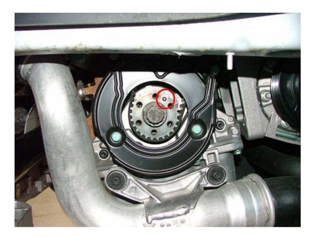
Note the indicated alignment pin. This must match with the recessed cavity on the back of the ECS Light Weight Crank Pulley, in order to assure proper, flush fitment.
