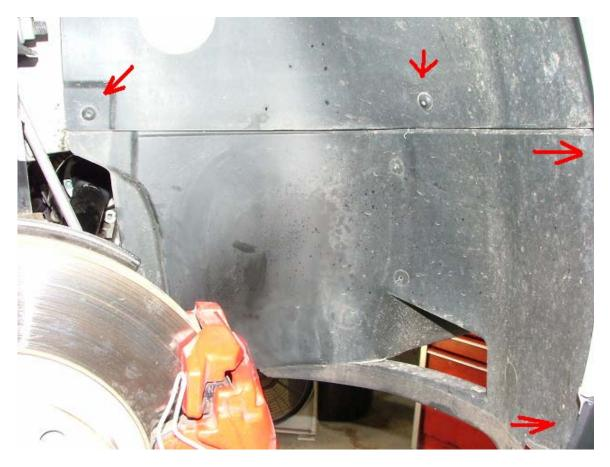
Remove the lower splashguard from the passenger side by removing the 11 T-25 pan head screws that hold it in place.
