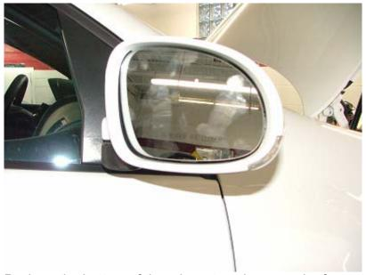
Push on the bottom of the mirror, to gain as much of a gap as possible at the top.
