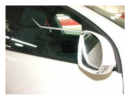
Gently work the top of the mirror out of the housing and work it loose. Pull the spade terminals off the back of the mirror and set it aside.
