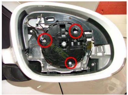
Remove the (3) T-10 Torx Fasteners from the mirror actuator unit. Unclip the actuator and set it aside.
