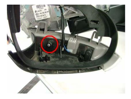
Remove the last T10 Torx, and remove the oem blinker assembly.
