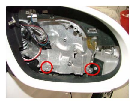
Remove the (3) circled T10 Torx Fasteners.
