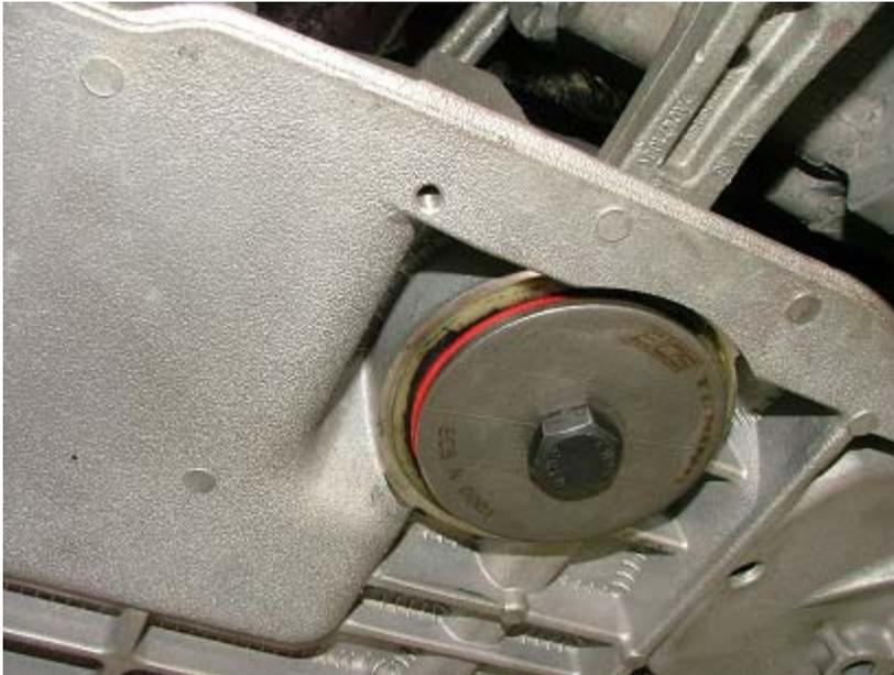
Insert the supplied 22mm bolt through the washers. Tighten to factory spec.
