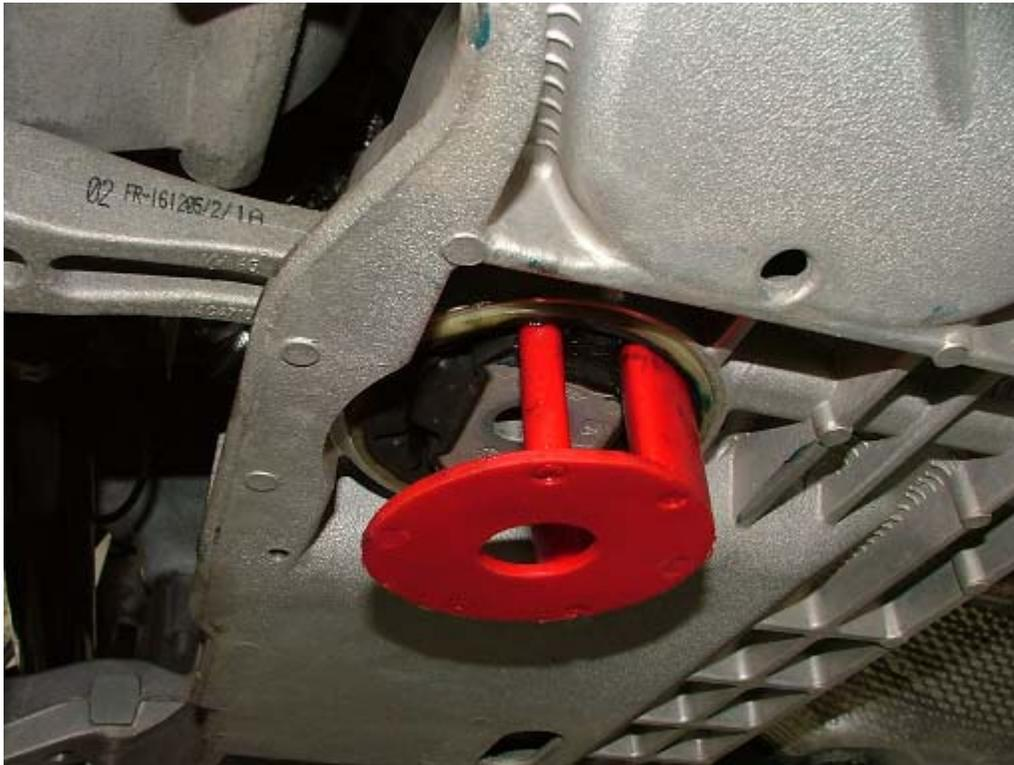
Apply grease to the urethane insert, and proceed to insert it into the mount. It's a tight fit and requires some effort to get it to seat completely.
