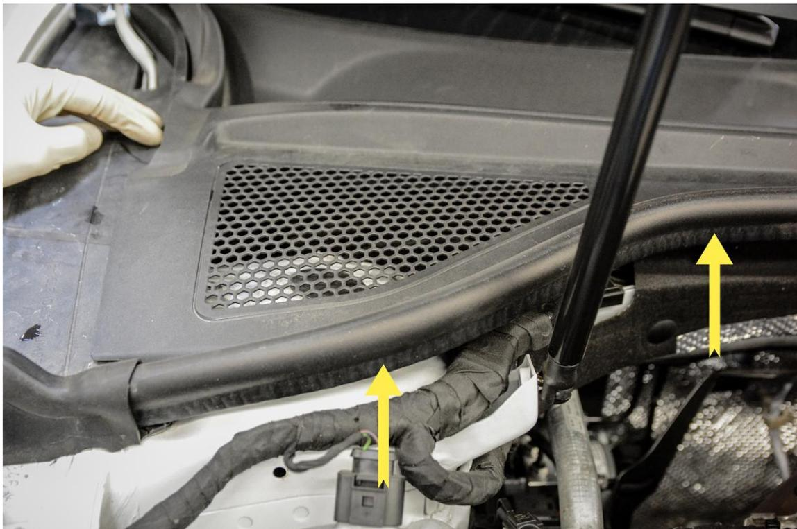
**Step 3** – With the weather stripping removed and the plastic cowl cover lifted, locate the bolt securing the dust shield to the strut tower.
