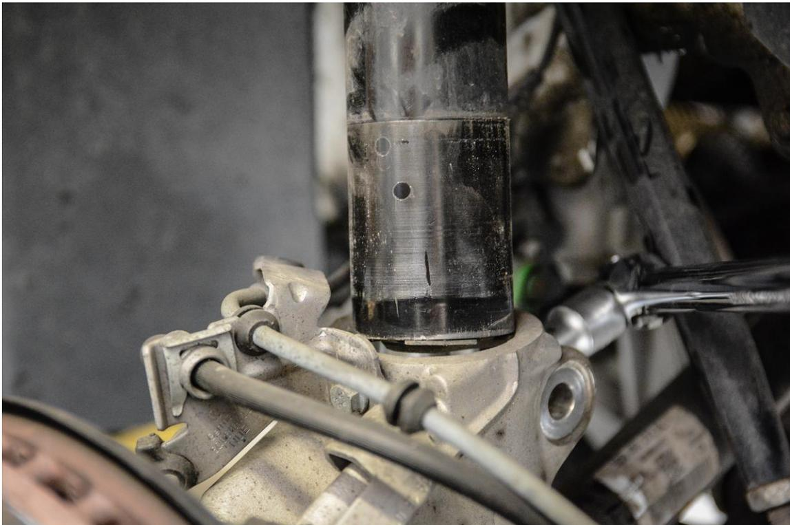
**Step 11** - Once the lower portion of the strut assembly is free from the knuckle, use a 13mm Socket to remove the 3 strut mount bolts.
