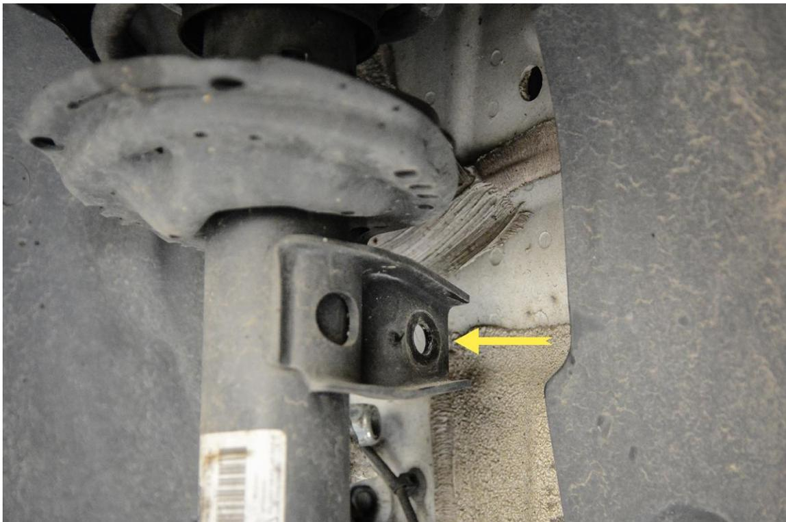
**Step 9** – Locate the bolt clamping bottom of the strut to the knuckle. Use a 14mm Triple Square and 18mm Socket to remove the nut and bolt from the knuckle assembly.
