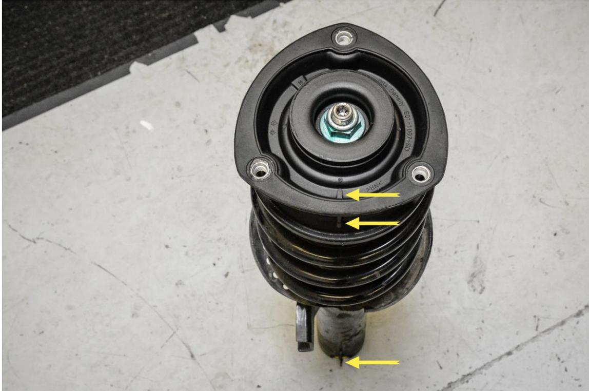
**Step 16** - Once upper strut nut is torqued, remove spring compressors and marvel at your work. You're ready to reinstall!!
