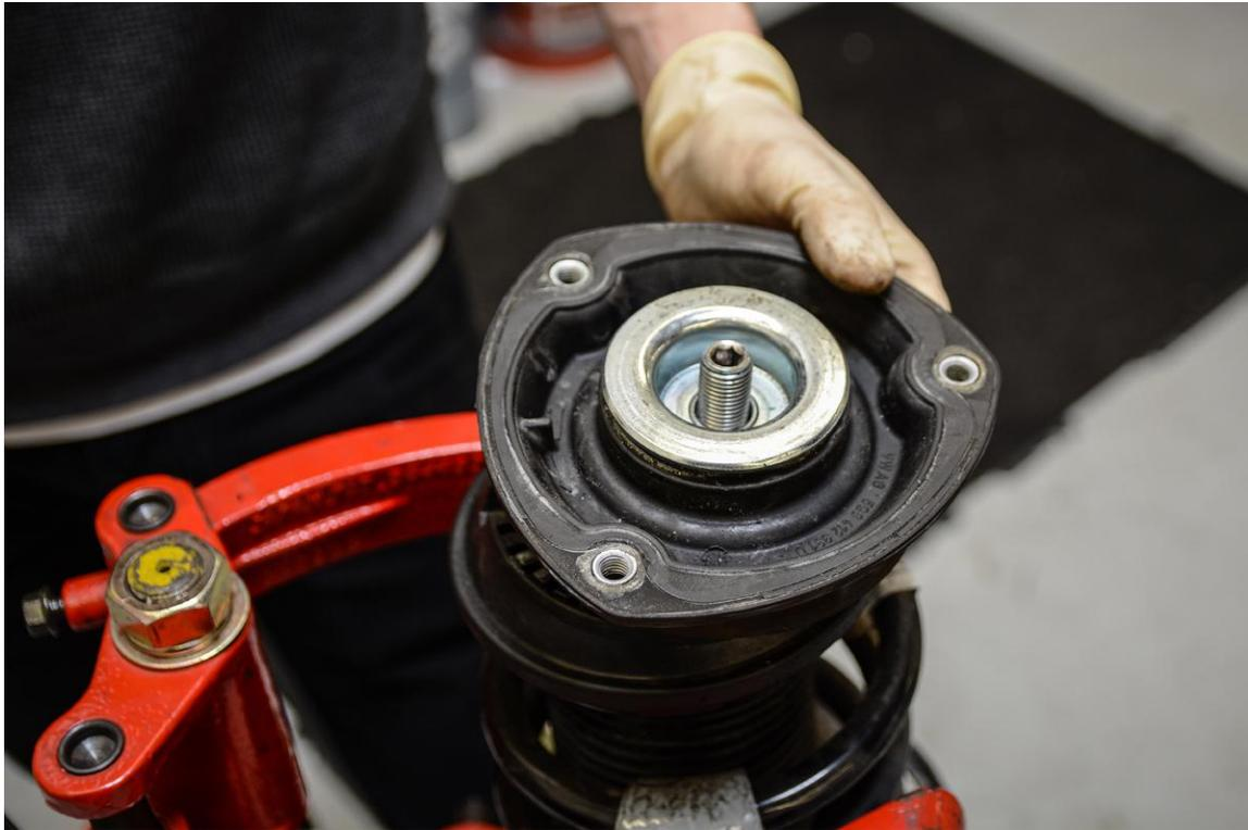
**Step 14** - Install new 034Motorsport Street Density Strut Mount and, if desired, new Strut Bearings. Locate tab on strut mount and align with recess in upper spring perch.
