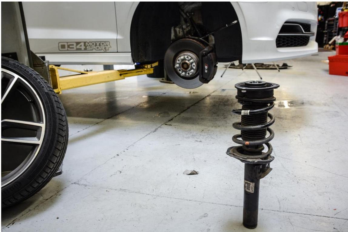
**Step 17** - Reinstall the strut assembly and loosely thread the upper 3 strut bolts into strut mount.
