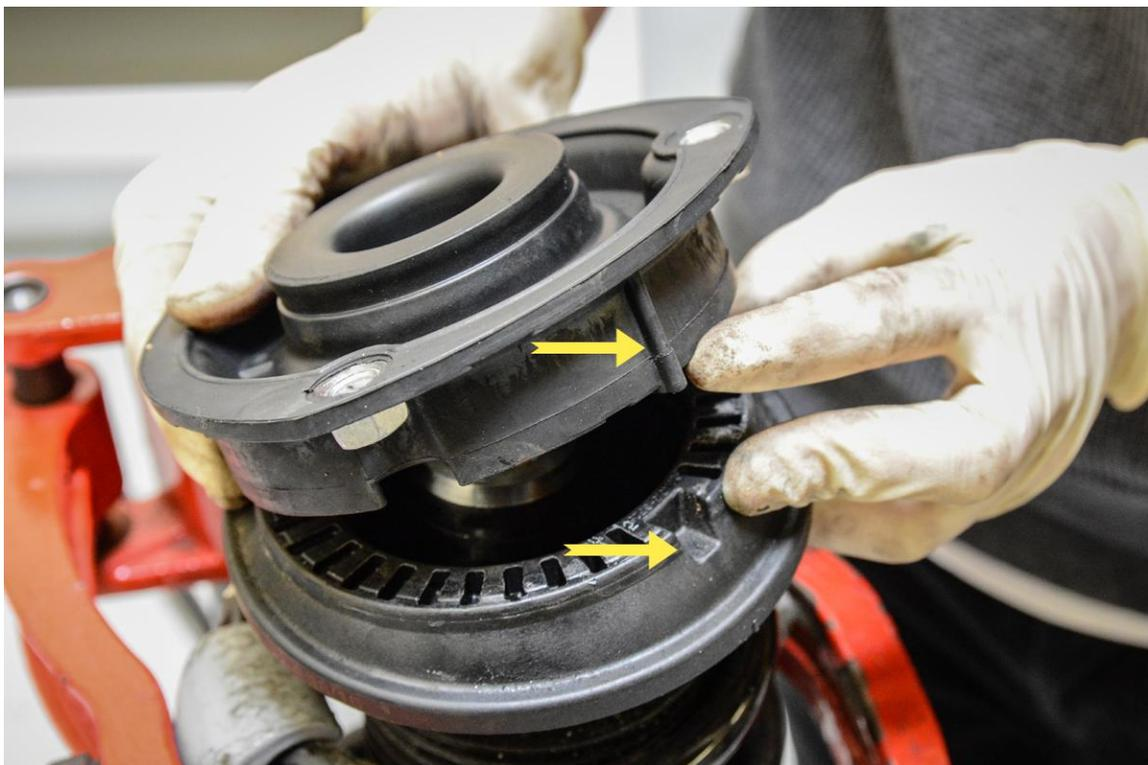
**Step 15** - Once all mounting tabs are aligned, install upper strut nut **using a 21mm (or 13/16" Standard) Spark Plug Socket and 7mm Allen**. Torque upper strut nut to 60 Nm. **Important:** For proper installation, the upper strut mount tabs must align with the tab on lower strut body.
