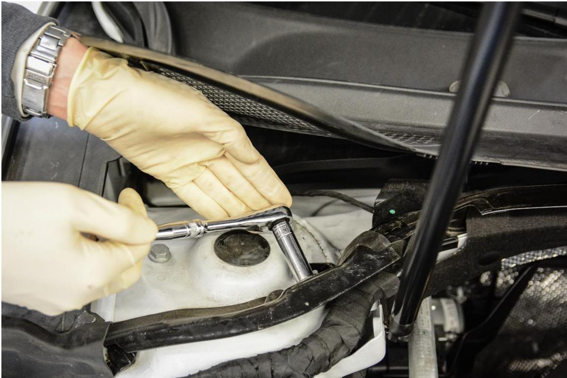
**Step 5** – With the dust shield out of the way, you'll notice the easy access to the 3 strut mount bolts for later.
