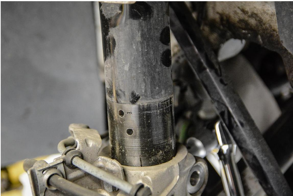
**Step 19** - Once strut assembly is bottomed out in the knuckle, reinstall bolt and nut using 14mm Triple Square and 18mm Socket respectively. Torque to 70 Nm + 90° turn.
