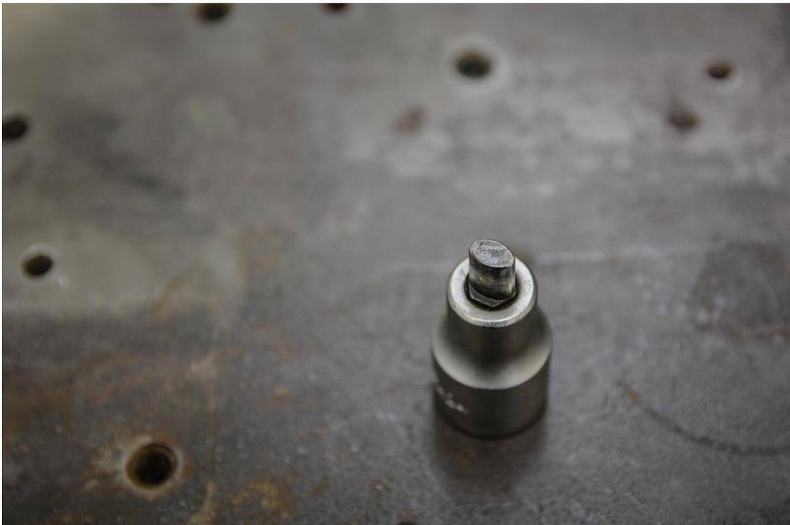
**Step 10B** – Once lower strut bolt and nut are removed, use a Spreader Socket to separate the strut housing from the lower knuckle. Spreader Socket shown inserted into lower knuckle below.
