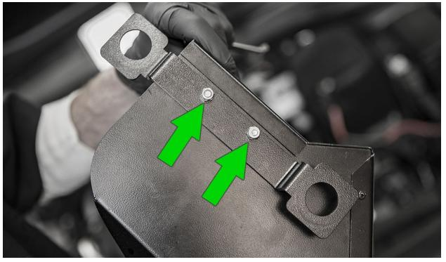
Press firmly to seat the included rubber grommets into the heatshield mount bracket. The flat side of the grommet with the IE part number will face down once installed.
