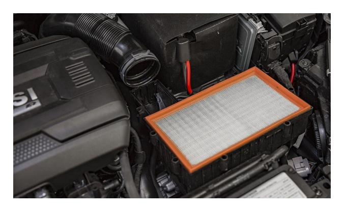
Remove the air filter by simply pulling it out.
