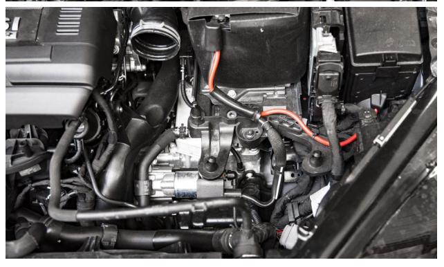
Loosen the hose clamp on inlet pipe turbo side using a screwdriver or 7mm socket. Fully remove the turbo inlet pipe and set the factory hose clamp off to the side, you will re-use it.
