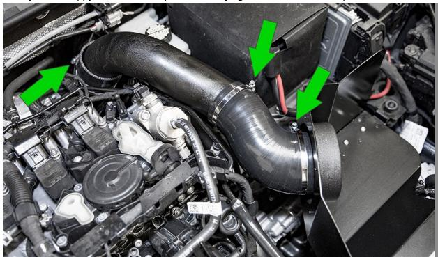
Install the factory vacuum hose onto the 90 degree barb fitting located on the underside of the silicone coupler.
