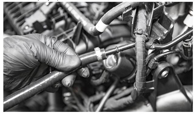
With the coolant line installed, tighten the pinch clamps using either the VW/Audi factory tool (if available) or wire cutters.
