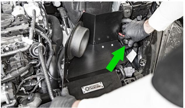
Pre-install the long-leg side of the aluminum pipe into the small diameter side of the IE silicone coupler with clamps. Do not tighten the hose clamps in this step.
