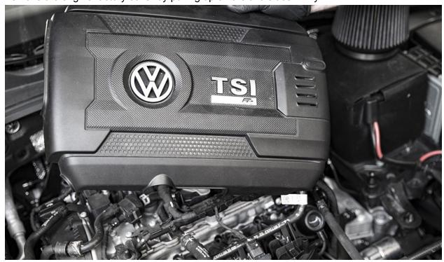
In the following steps you will be removing a factory coolant line. This line is located just in front of the removed intake box attached to the upper radiator hose.
