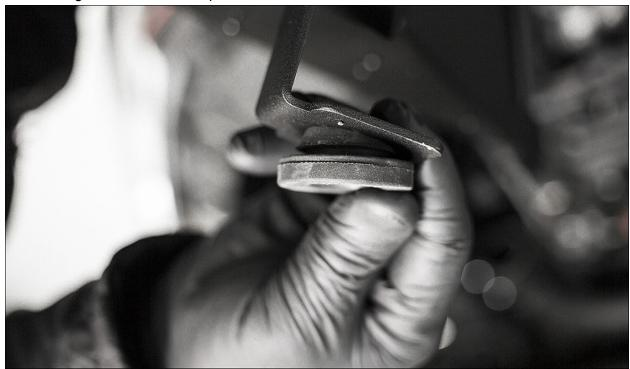
Remove the engine factory cover by pulling up on the two sides firmly.
