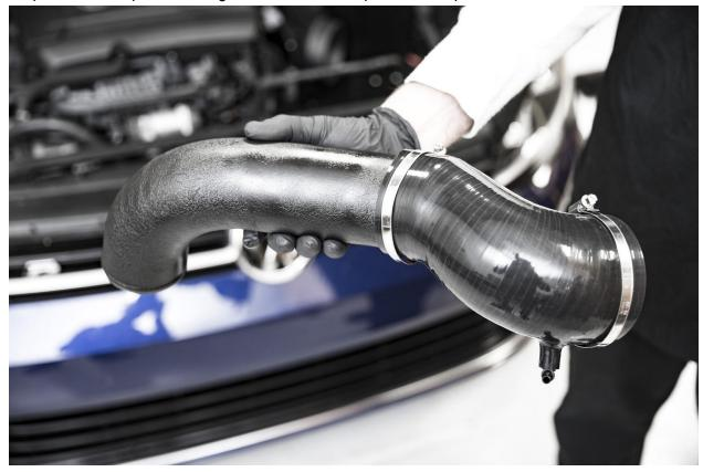
Place the intake pipe and coupler in place. Insert the intake pipe into the installed turbo silicone coupler and connect the opposite side to the heat shield. Re-align the silicone coupler and turbo
