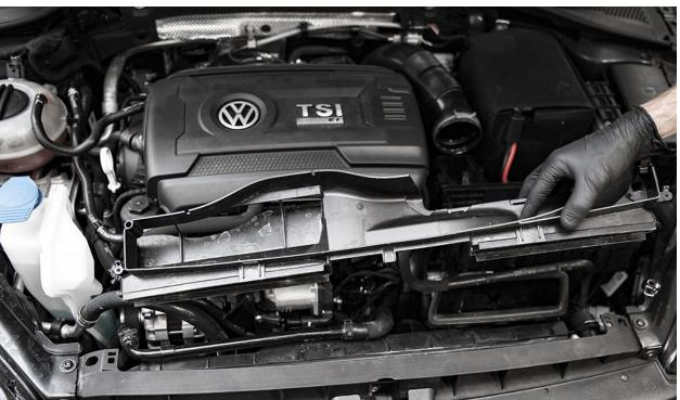
Carefully pull up on the factory lower airbox to release it from the battery tray and remove it. The airbox is held down by 3 rubber grommets securing it to plastic posts.
