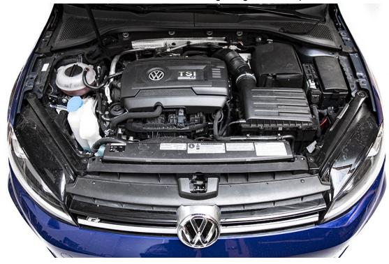
Start the installation procedure by loosening the eight T25 bolts from factory airbox lid. These do not fully remove, just loosen them until they are spinning freely.
