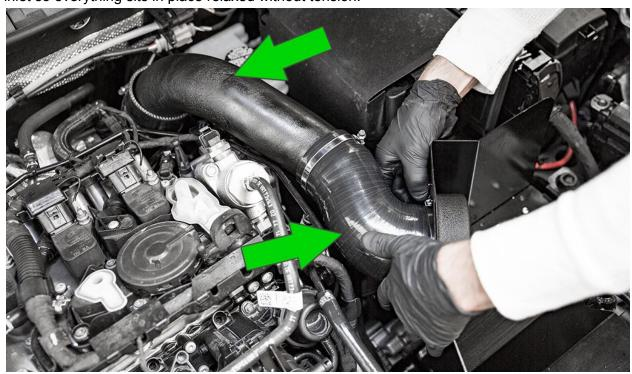
Once you are happy with the intake position, firmly tighten all the hose clamps.
