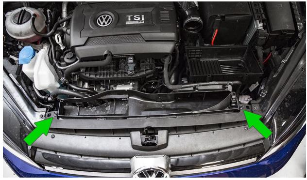
Remove the far portion of the intake inlet box located on the driver's side by pulling up on the lock tab.
