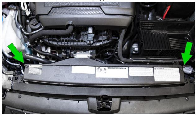
Pull to release the tab on the back side of the upper airbox inlet cover, then fully remove it.
