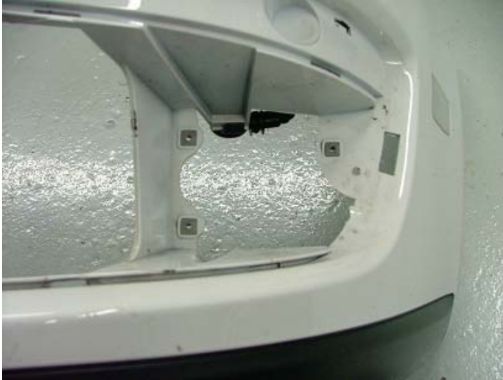
Speed clip inserts installed.
