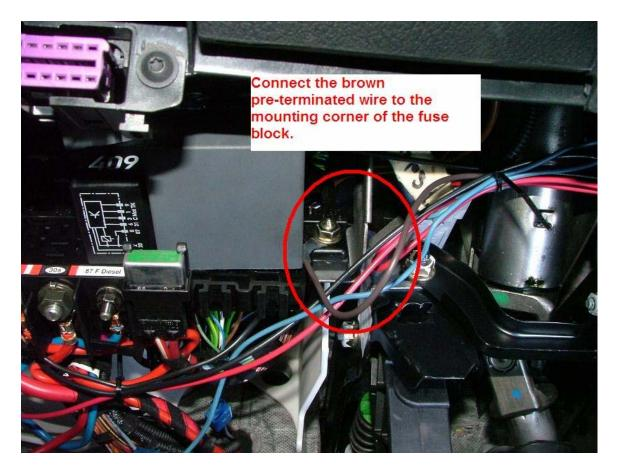
To get our proper ground, a good ground is the corner of the fuse block mounting point, under the 10mm securing nut.
