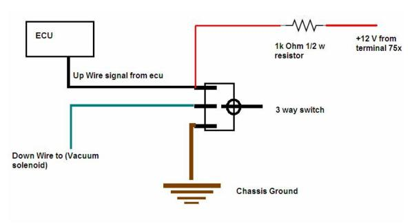
The schematic of the harness is as follows.
